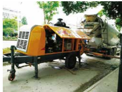
HBT6013V 江苏徐州 HBT6013V trailer-mounted concrete pump in Xuzhou, Jiangsu
